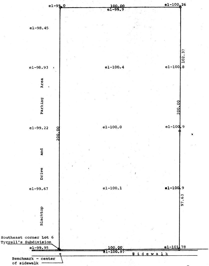
Benchmark - center of sidewalk Assumed elevation = 100.00
